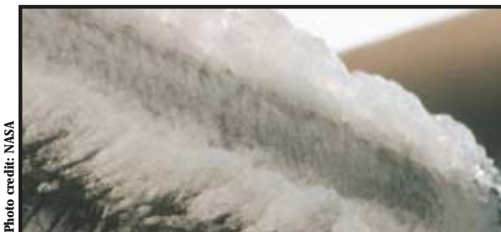
In-flight wing leading edge ice formation
