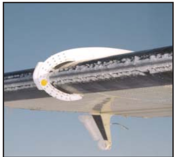
Mixed ice formation on wing leading edge
