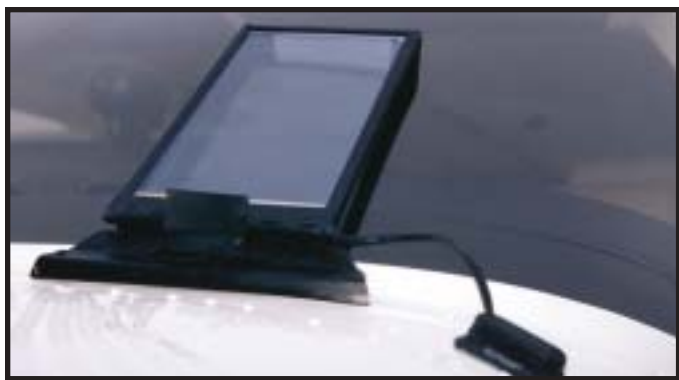
Electrically heated windshield
